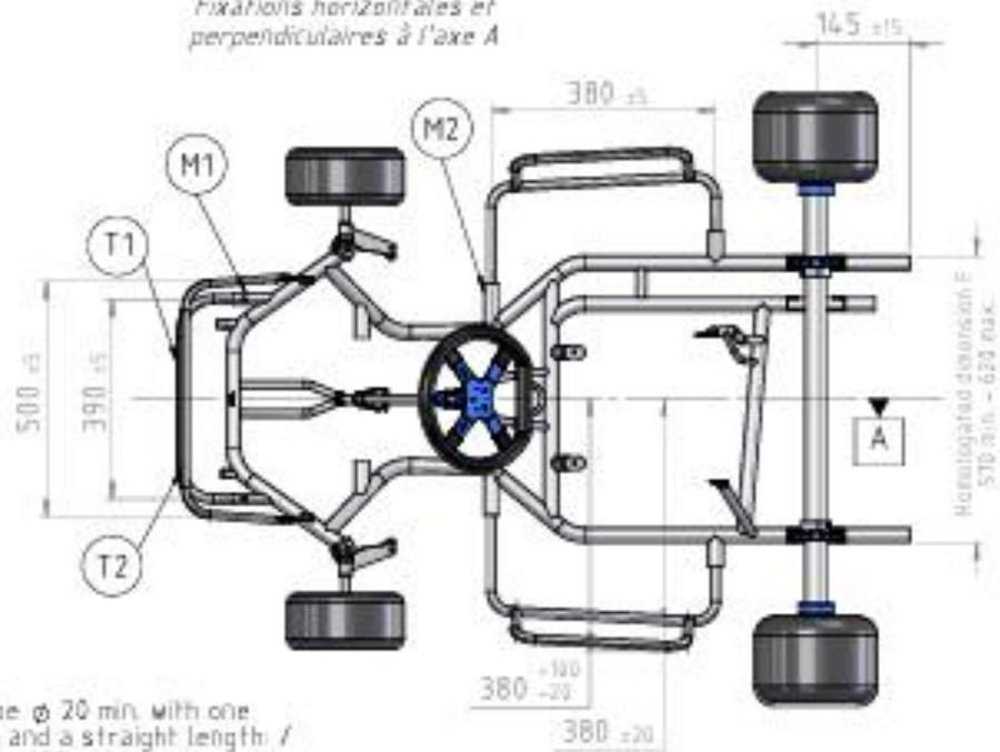
T1: Lower tube  $\phi$  20 min. with one constant radius and a straight length: /
