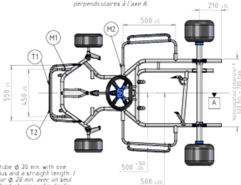
T1: Lower tube  $\phi$  20 min. with one constant radius and a straight length /
